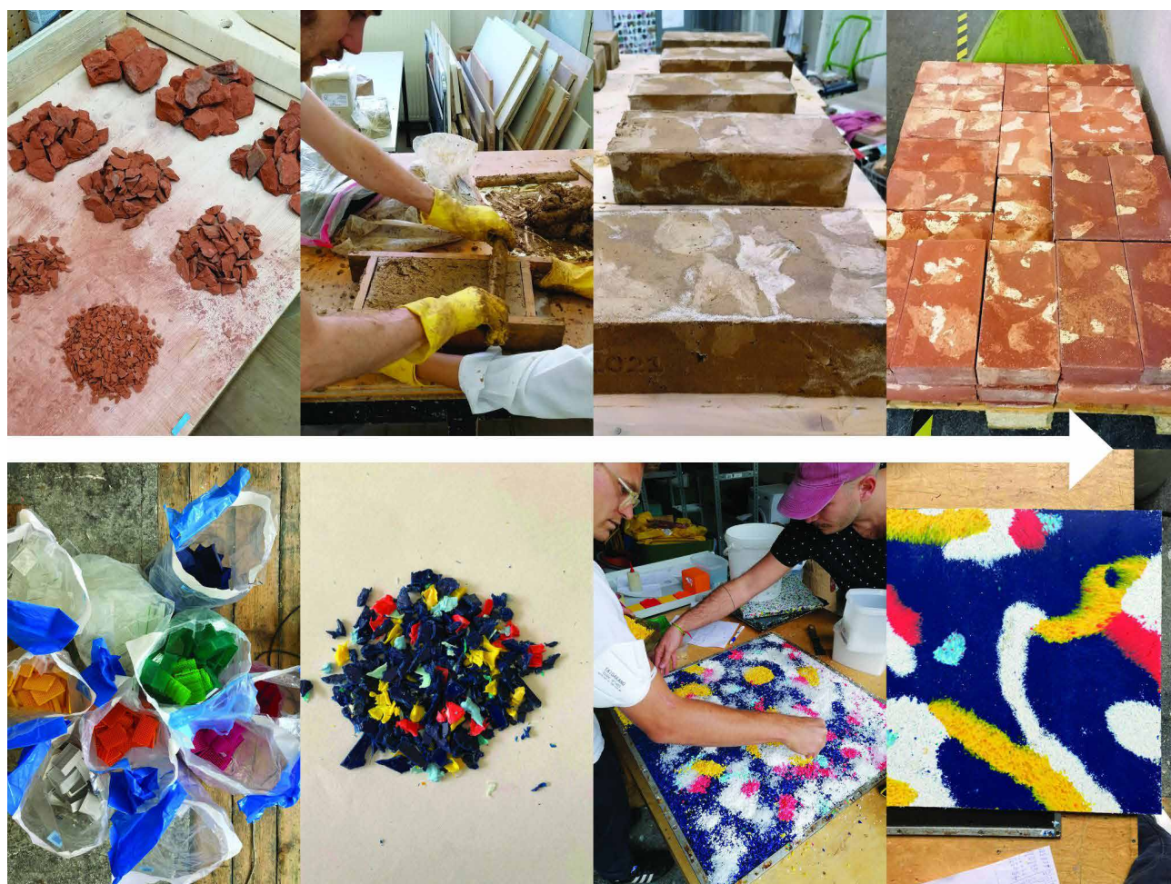
Figure 8. When reuse was not possible, materials were recycled, such as deteriorated bricks and plastic waste, ensuring zero on-site waste generation. © Social Design Studio.
